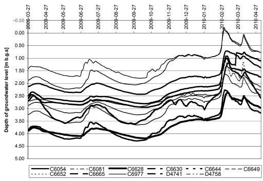
Fig. 5. Groundwater level depth at 11 piezometers for the period 27 March 2009 to 5 May 2010.
